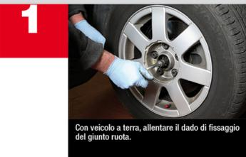
With the vehicle on the ground, loosen the wheel joint fixing nut.
