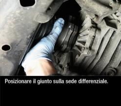
Fit the joint in the differential housing.
