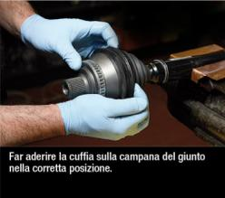
Fit the boot correctly onto the joint bell.
