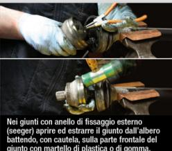
For joints with external fixing washers (seeger) open and extract the joint from the shaft, carefully beating the front of the joint with a plastic or rubber hammer.
