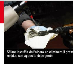
Slide the boot off the shaft and remove any excess grease with suitable detergent.
