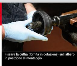
Fix the supplied boot onto the shaft in the assembly position.
