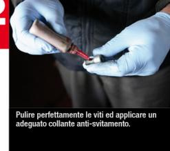
Perfectly clean the screws and apply a suitable locking glue.
