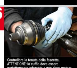
Check the clip seal. ATTENTION: the boot must adhere perfectly and not turn.
