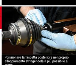
Fit the rear clip in its housing and tighten it by hand as far as possible.
