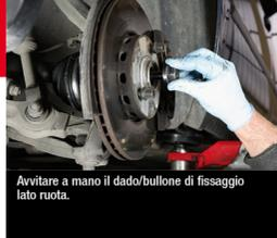
Screw the fixing nut/bolt onto the wheel side by hand.
