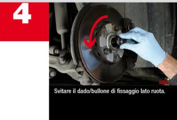
Unscrew the fixing nut/bolt on the wheel side.
