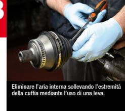
Remove the air from inside, by lifting the end of the boot with a lever.
