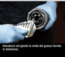
Put half of the supplied grease into the joint.
