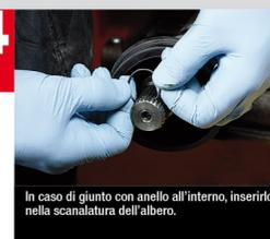
If the joint has an internal washer, fit it into the groove on the shaft.
