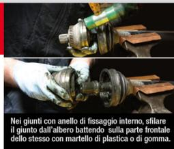
For joints with internal fixing washers slide the joint of the shaft, beating on the front of it with a plastic or rubber hammer.
