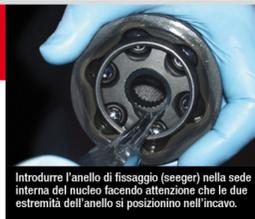
Fit the fixing washer (seeger) into the inner seat on the core, taking care that the two ends of the washer are fitted in the notch.
