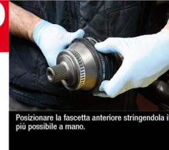
Fit the front clip and tighten it by hand as far as possible.
