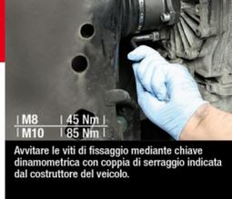
Tighten the fixing screws using a dynamometric spanner, with the torque given by the vehicle manufacturer.
