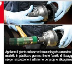
Put the joint onto the groove and push it down, with the help of a plastic or rubber hammer, until the fixing washer or seeger washer is positioned in its housing.
