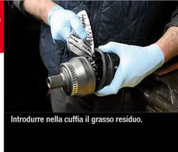
Put the remaining grease into the casing.
