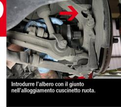
Fit the shaft and joint into the wheel bearing housing.
