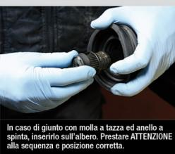
If the joint has a cup spring and circlip, fit it onto the shaft. Pay ATTENTION to the correct sequence and position.
